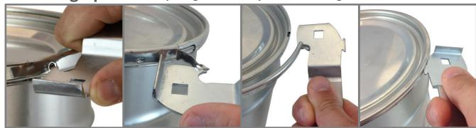
Place the point of the beak firmly into the hole of the latch ring
